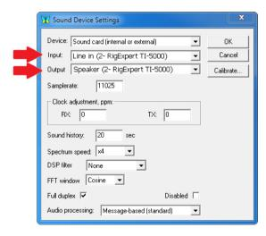
Select RigExpert TI-5000 as both Input and Output, then check other settings and finally press OK to apply new settings.
