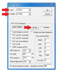
In the Serial port window, select a serial port number for the CAT system. Select a baudrate and a number of stop bits according to the user's manual of your transceiver. Press OK to close this window, and then review other settings in the PTT&CAT dialog. Finally then press OK to finish.
