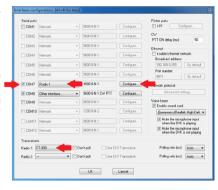
Select baudrate and the number of stop bits according to the user's manual of your transceiver. Click OK to continue.
