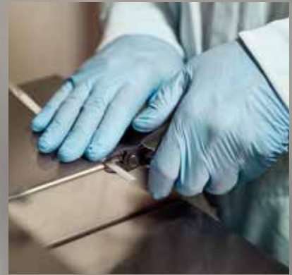
8150M2 cutter used to trim multiple stents thanks to the modified hardened cutting heads.
