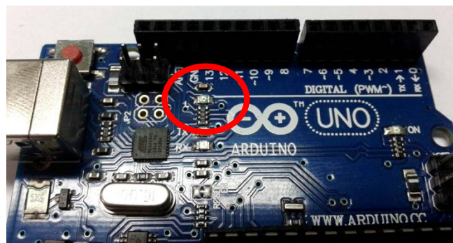
Figure 8. The position of LED L on Arduino Board circuit
