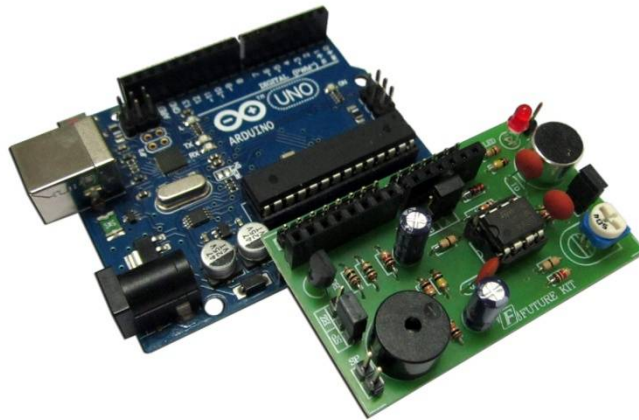
Figure 9. Connecting FK1419 board with Arduino UNO R3 board
